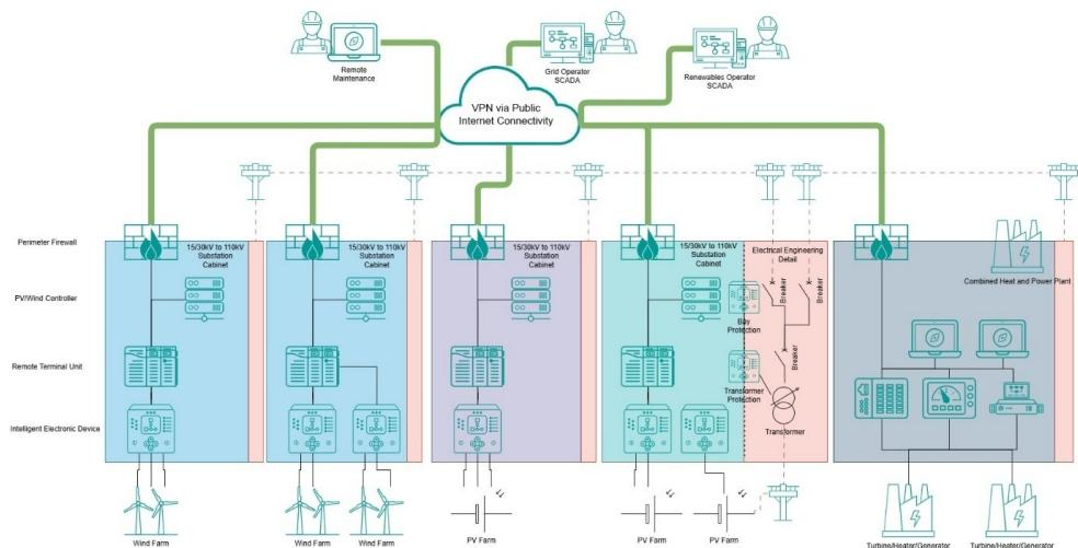
RTUs standardize how distributed sites interface with control centers, enabling operators to manage large numbers of remote facilities from a single SCADA system. Within these installations are systems often specified by manufacturers or chosen by system integrators, leading to significant variations in implementation. The technology may be similar across sites, but configurations and applications differ.
